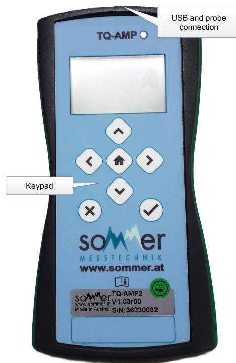
Figure 3 After connecting the USB cable power supply the batteries are charged
