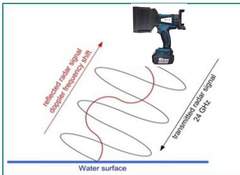
Figure 1 Principle of flow velocity sensor
