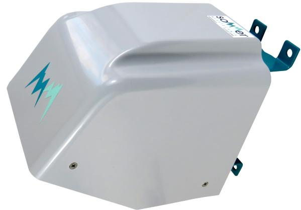
The RG-30+ radar sensor is a measurement device for the contact-free determination of the flow velocity of open rivers and channels. The sensor detects the surface flow velocity by the principle of the Doppler frequency shift.
