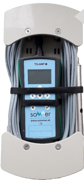
TQ-S Heavy Duty Version: with handy cable-spool and probe
