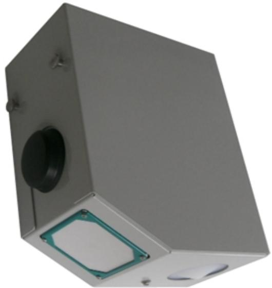
The RQ-30 ADMS is an all-in-one discharge measurement system, suitable for spot-measurements, temporary applications or stationary long-term installations. It contains the contact-free flow velocity and water level sensors of the RQ-30, Data logger and batteries and applies the same algorithms to compute the water discharge.
