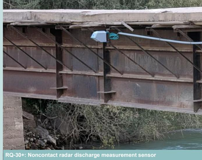
RQ-30+: Noncontact radar discharge measurement sensor
