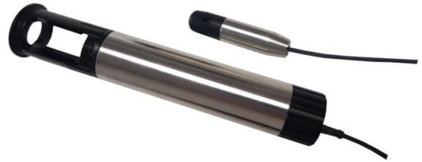
The PD-Mini data logger is a compact device for level monitoring of groundwater wells. Besides water level it acquires air pressure, temperature and battery voltage. The recorded data can be downloaded by a 433-MHz radio USB adapter (available as accessory) and a support software that exports measurement data as Excel files.
