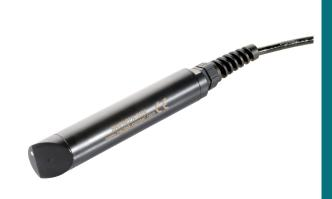
The measurement principle of the SOMQUALITY-NTU turbidity sensor is based on infrared light scatter at an angle of 90°. Thanks to the measurement at a wavelength of 880 nm and the wide detection range of 0 to 4'000 NTU, the sensor can be used in varous water and wastewater treatment applications. Apart from turbidity, the SOMQUALITY-NTU also measures the medium temperature and the suspended solids content.
